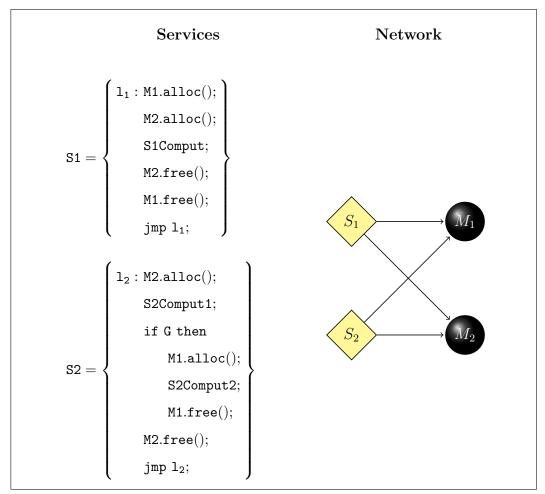
Fig. 3. A simple system with two services and two resources
