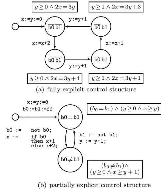
Figure 1. Associating invariants to control location. The boxes formula give the invariant computed for each location with a linear relation analysis
