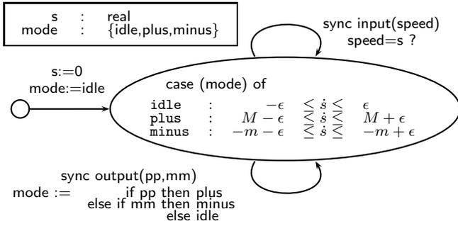
(a) Environment: disk motor device emits the speed of the disk on channel input and reacting to the controller (channel output)
