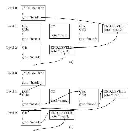
Fig. 3. Cluster code and the linked list pointers. (a) At the beginning of a cycle. (b) After executing sched3a, sched1b, and sched4.
