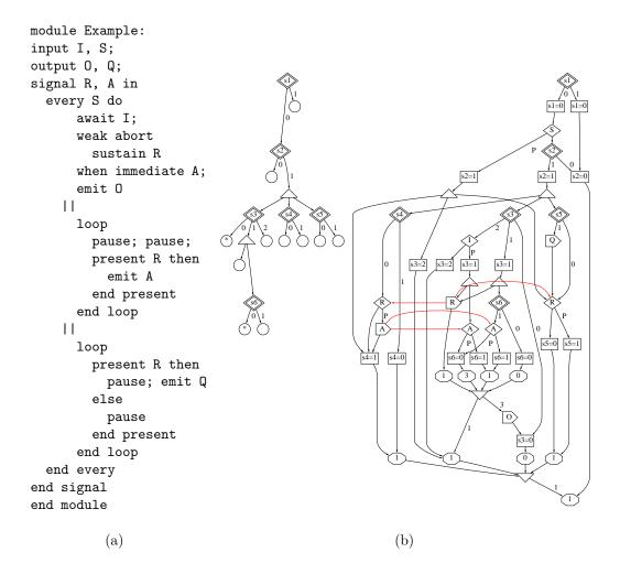
Fig. 1. An Example. (a) A simple Esterel module modeling a shared resource. (b) The (simplified) GRC graph, consisting of a selection tree and a control-flow graph.
