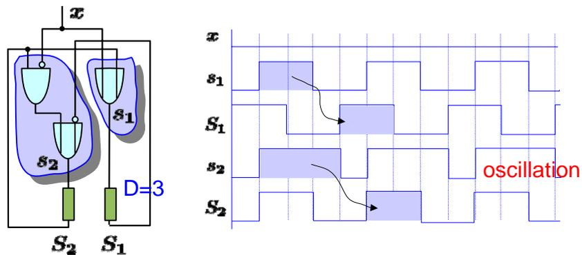
Non-inertial (UN-) delays **permit oscillation** as predicted by ternary simulation.
